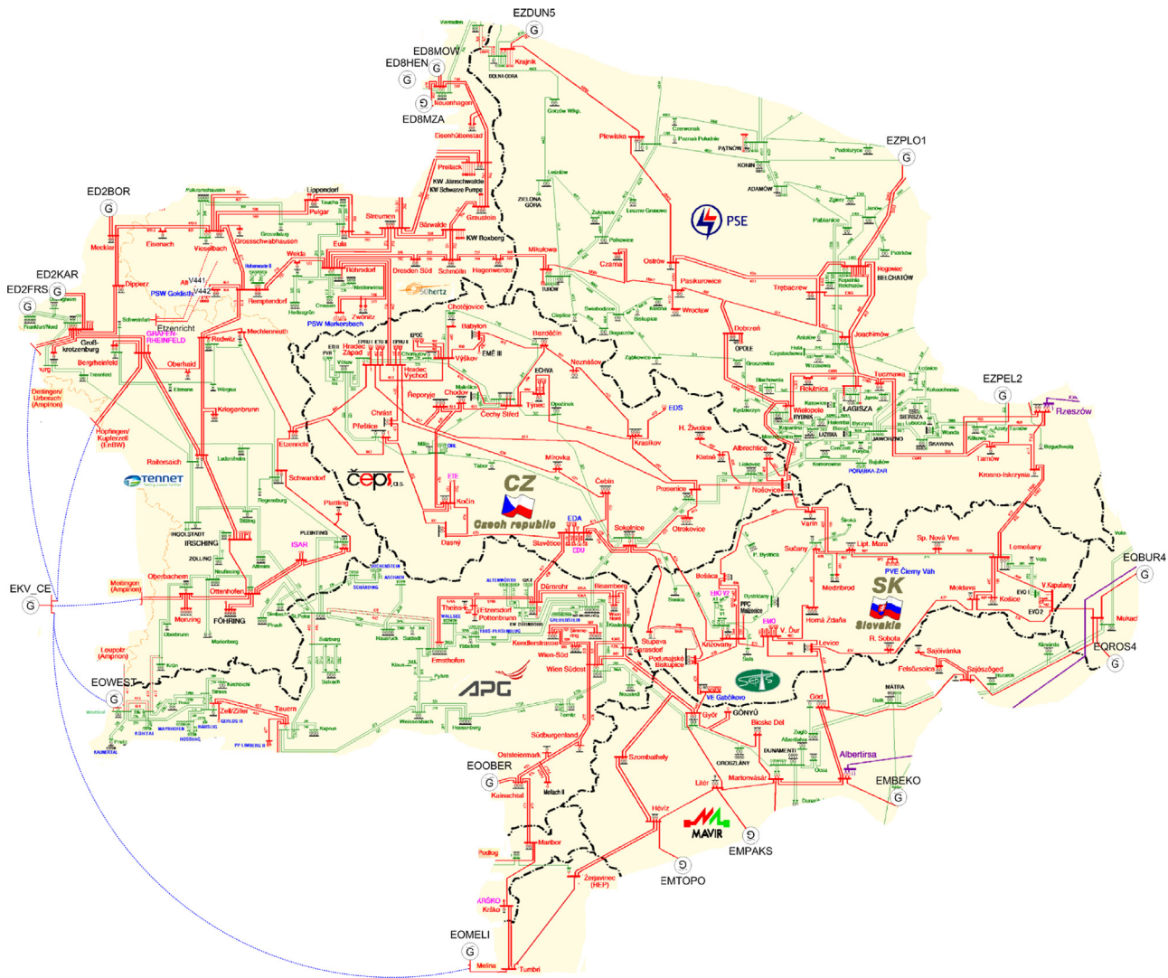
Fig. 9. One-line diagram of the observable area as a part of the central European transmission system.
