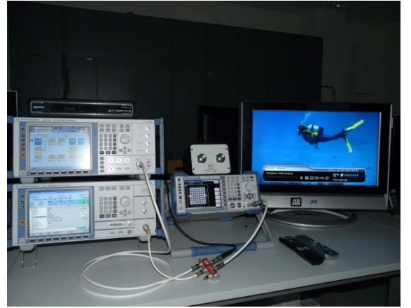
Fig. 3. Realized laboratory workplace for measuring the interaction between DVB-T/H and LTE networks (R&S SMU200 LTE signal generator, R&S SFU DVB-T/H transmitter, R&S ETL TV analyzer, Set-Top-Box and TV screen).
