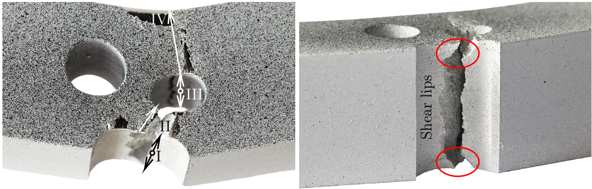
Figure 4.6: Fractured specimens after the three-point bending test [99]
