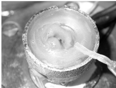
Fig. 4. Specimen of the small intestine embedded in agar; the cup is placed on the Peltier-cooled holder.
