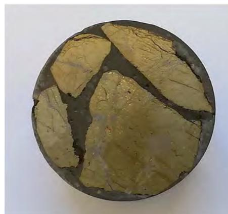
Fig. 1 The rocks were placed into resin to form a sample, and its surface was polished.
