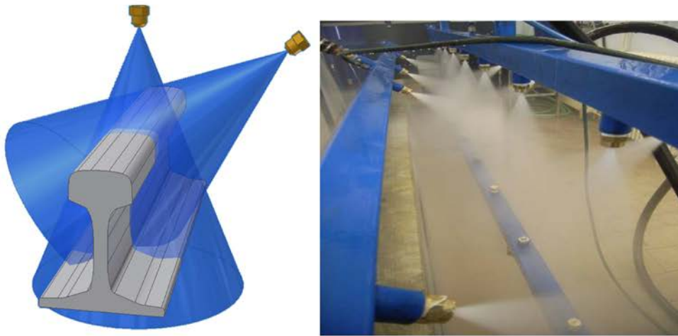
FIGURE 3. Numerical modeling of positioning nozzles for cooling of rails and spraying cooling section
