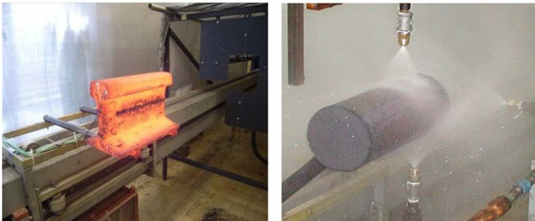
FIGURE 4. Samples of rail and tube are positioned on movable trolley at linear test bench and runs through cooling sections
