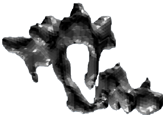
Fig. 3 - 3D reconstruction of a shrinkage pore using X-ray computed tomography.
