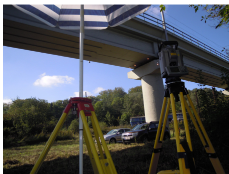
Obr. 102 – monitoring stanicí Trimble S8
