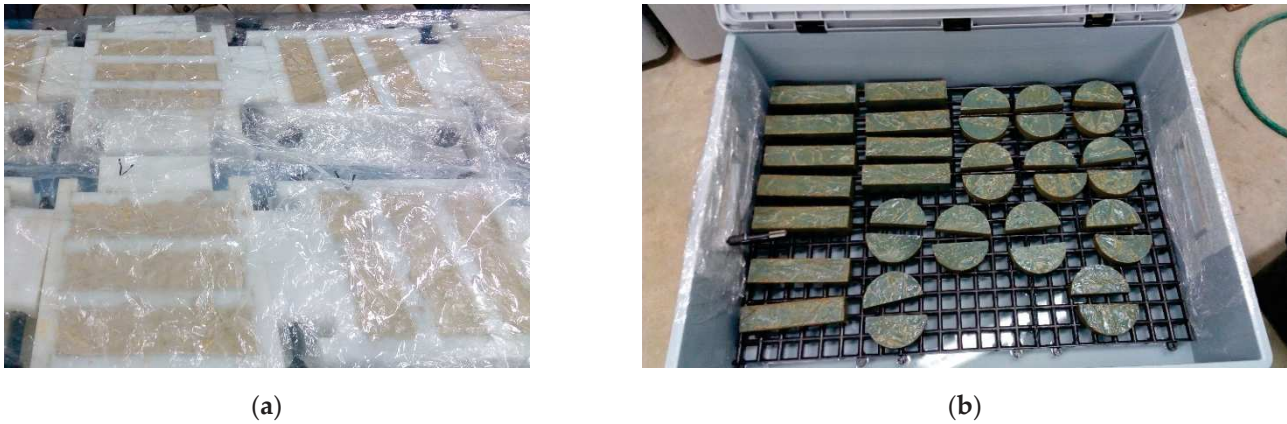
Figure 3. Manufactured test specimens covered with a stretch PE foil (a); test specimens after demolding prepared to storage in a closed box with RH > 95% (b).
