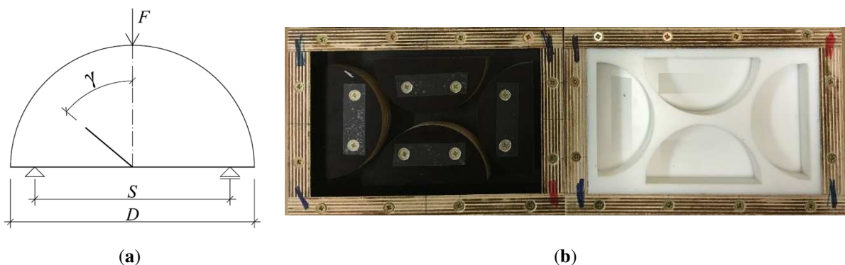
Figure 4. Three-point bending fracture test configuration of a selected semi-circular disc specimen with an inclined initial notch (a); and a special mould (b).
