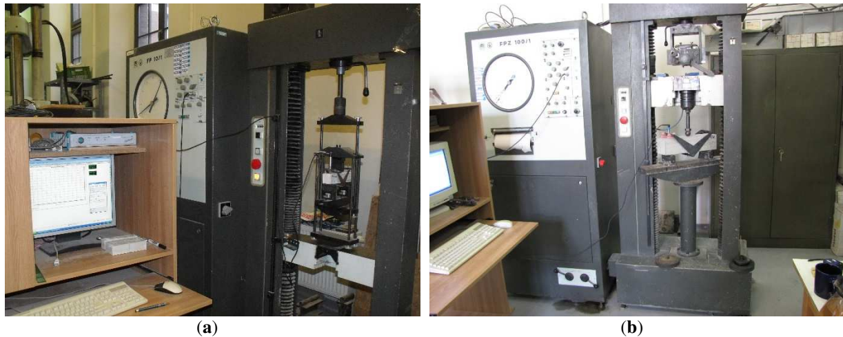
Figure 5. The testing machines used for fracture tests: Heckert FPZ 10/1 (a), and Heckert FPZ 100/1 (b).
