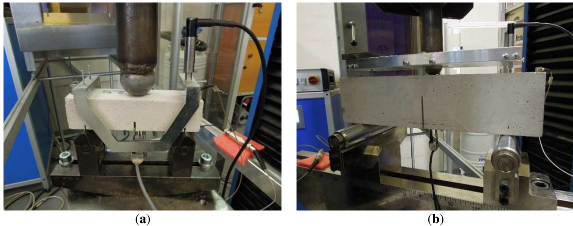
Figure 7. Detail of the test measuring frame: placed on the specimen (a), bedded on the upper surface of specimen (b).
