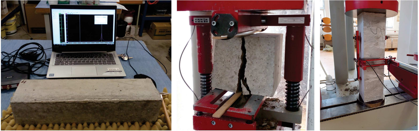
FIGURE 5 Measurement of the natural frequency of longitudinal vibrations (left), splitting tensile test (middle), and static modulus of elasticity test (right)
