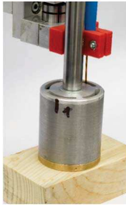
Figure 15. Testing device for the measurement of the overall response time of the damping force.
