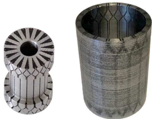
Figure 22. The printed bobbin and outer cylinder with plastic material in the isolation distances.
