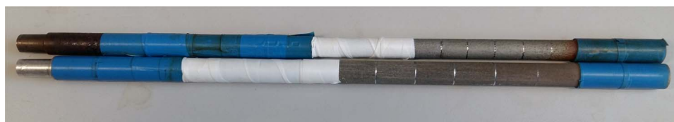
Fig. 2. Partly taped and partly exposed mild steel (upper) and aluminium (lower) electrode with clearly distinct sections.
