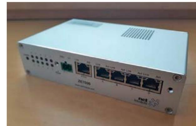
Thanks to the use of the FPGA technology and specially designed hardware architecture, the probe allows to precisely capture network communication not only based on identifiers from the network layer but also using identifiers from the application layer. The results of this project serve primarily to the police and other State security forces as a tool in the fight against cyber criminality.
