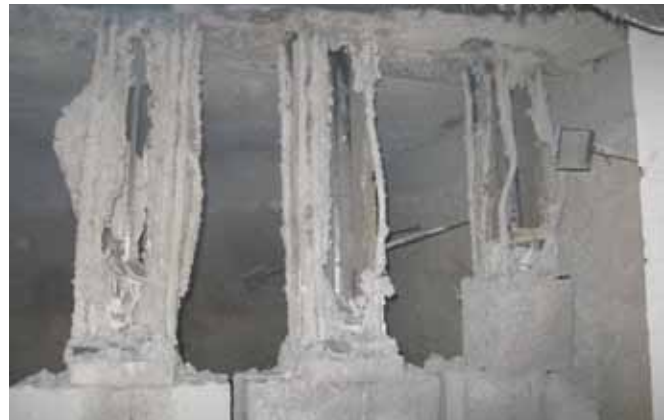
The composite reinforcement in testing frames after a fire test – a view of the furnace
