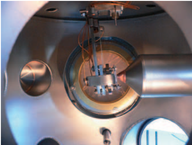
A sample holder in front of a device for mass spectroscopy of evaporated atoms (Laboratory of surfaces, thin layers, and nanotechnologies, Institute of Physical Engineering of the BUT Faculty of Mechanical Engineering)
