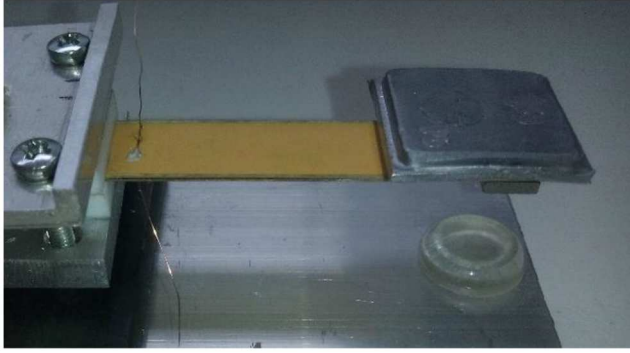
Fig. 3. Example of the real energy harvester with a tip mass.
