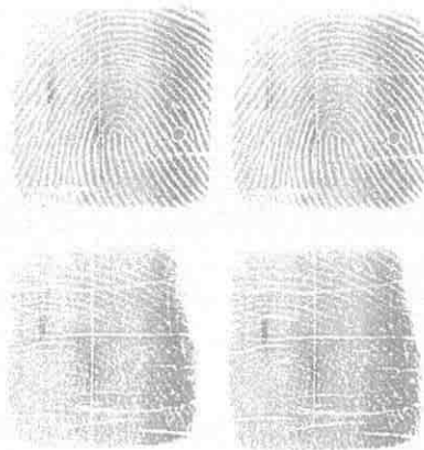
Fig. 4.5: The top pair shows captures of an artificial finger acquired 0 and 5 second apart and the bottom pair shows the same for a cadaver finger [48].
