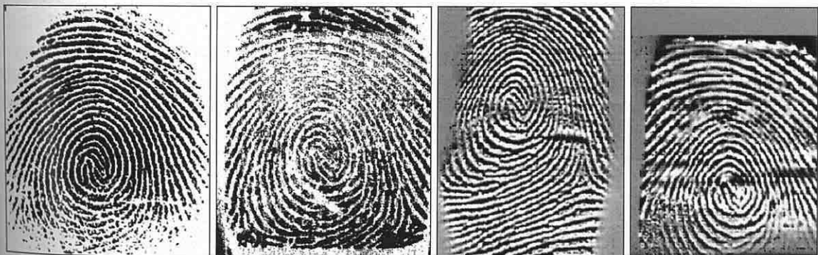
Fig. 4.42: Fingerprint images [Dra33] (from left to right): a) real finger captured by an optical sensor; b) fingerprint stamp captured by an optical sensor; c) real finger captured by a thermal sensor; d) fingerprint stamp captured by a thermal sensor.
