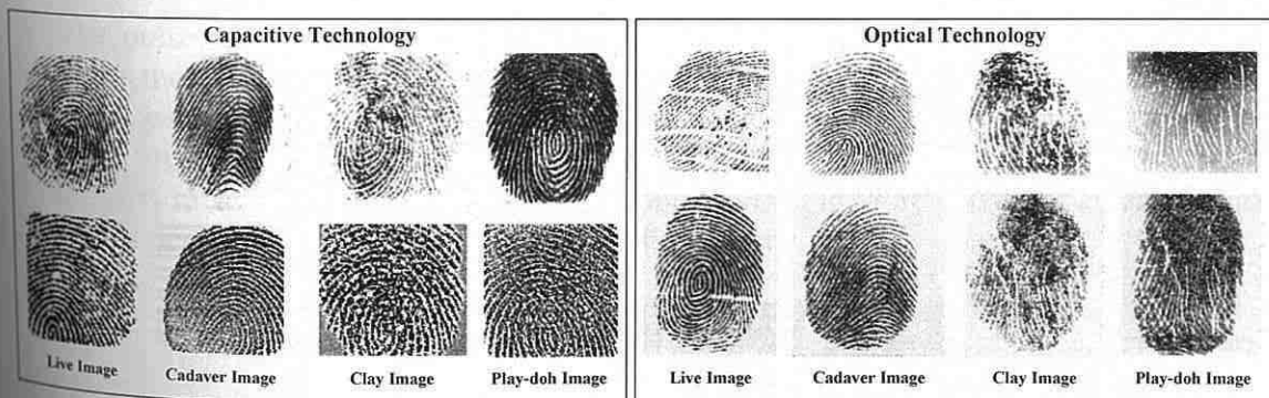
Fig. 4.36: Measurement of fake fingers using different scanner technologies [88].
