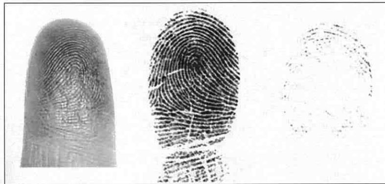
Fig. 4.14: Index finger with newsprint to demonstrate the finger contamination (from left: contaminated original, ultrasound image, optical image) [95].
