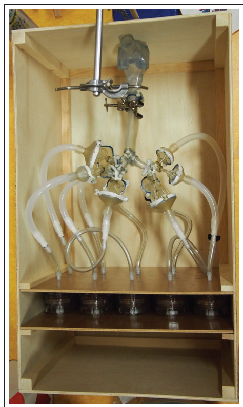
Figure 3. A photograph of the model in a box before the connection of hoses to flow meters.
