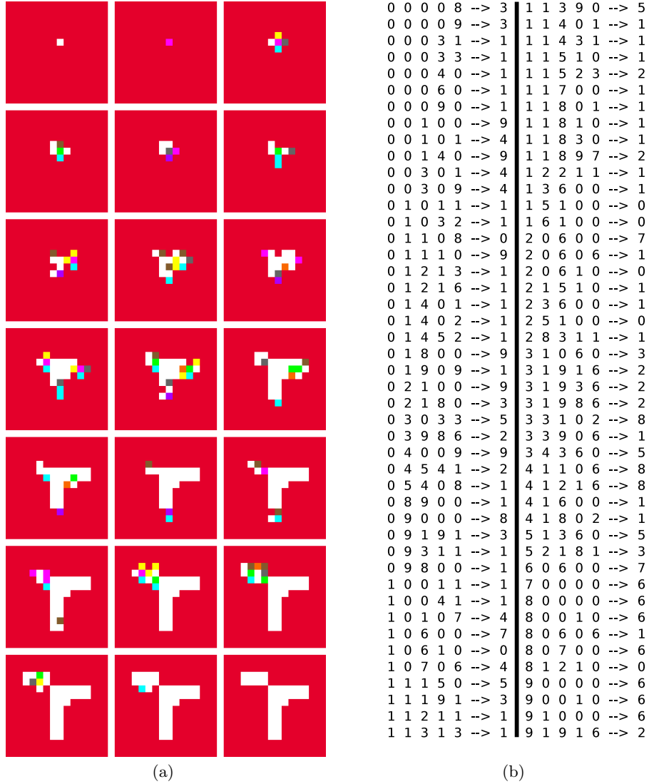
Fig. 10. Example of an evolved CA for the development of the BUT logo. The initial state consists of a single cell state 1, the other cells possess state 0. (a) The sequence of CA states producing the final pattern (ordered from left to right and top to bottom). (b) The appropriate transition rules for this CA.
