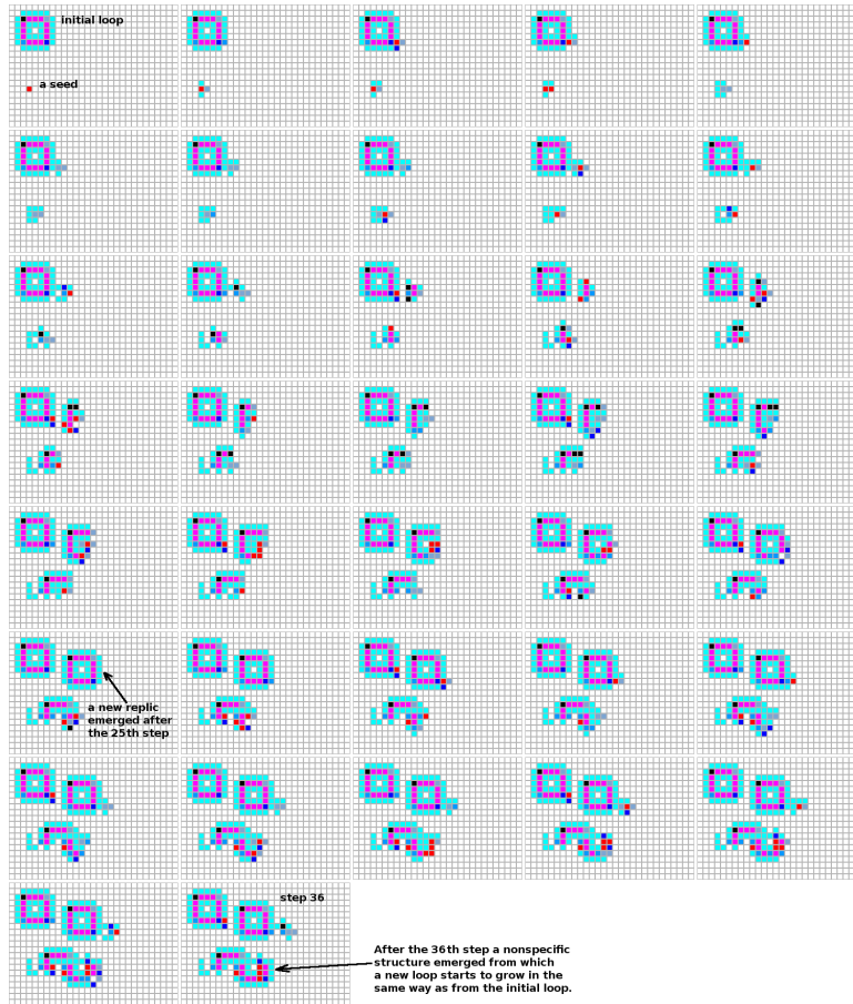
Fig. 6. Part 1 of the replication according to the transition function from Figure 5. The sequence of steps reads from left to right and top to bottom. The development shows a replication of the initial loop (the upper part of each step) and a growth of a non-specific structure from a seed allowing to create the loop autonomously (the lower part of each step). The seed is represented by a cell in state 7.
