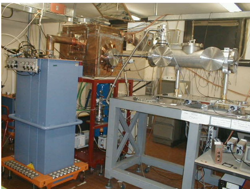
Figure 20. The capillary-discharge based soft X-ray laser at the University of L'Aquila, Italy [108].
