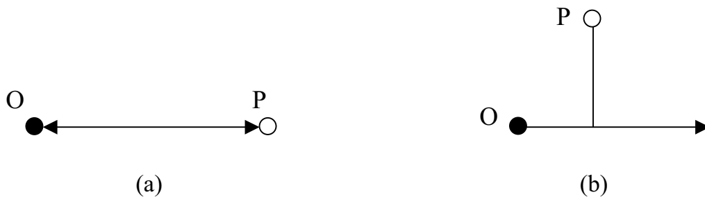
Fig. 1.1. (a) Measurement setup for longitudinal velocity measurement. (b) Measurement setup for transversal velocity measurement.
