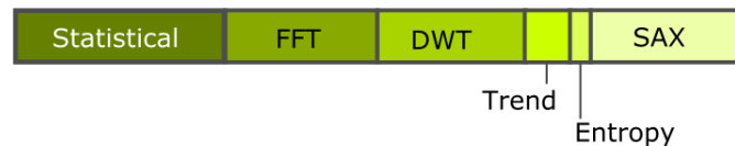
Figure 10: Time-lapse feature extraction from the univariate time series. Extracted time-lapse features are assembled into a partial time-lapse feature vector. Individual segments represent the group of time-lapse features obtained by the particular extraction technique. The length of the segments indicates the approximate number of extracted time-lapse features for the particular group.
