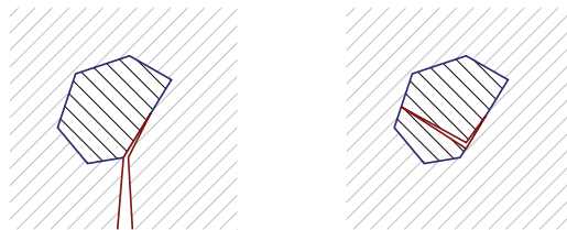
Figure 18: Crack propagating through the inclusion/matrix interface. On the left-hand side the crack originates in matrix. On the right-hand side the crack originates in the inclusion.
