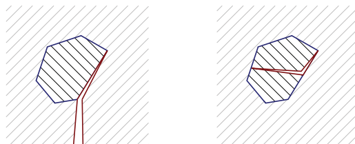
Figure 19: Crack propagated to the end point of inclusion/matrix interface. On the left-hand side the crack originates in matrix. On the right-hand side the crack originates in the inclusion.
