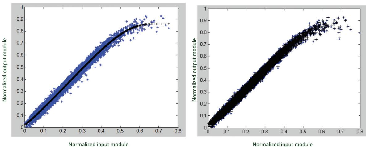
Figure 10: Memory polynomial model fits to measured PA signal:  $K=7, Q=0$  (left) and  $K=3, Q=23$  (right)
