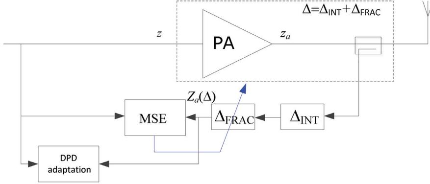
Figure 14: Block schematic of time-delay adjustment
