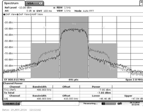
Figure 11: Power spectrum for example PA in 800 MHz band excited with 16QAM signal: TR2 - black curve denotes LUT DPD, TR3 - green color is PA without DPD, and TR4 - orange trace is DPD with orthogonal memory polynomial with orders  $K = 7$  and  $Q = 3$ .
