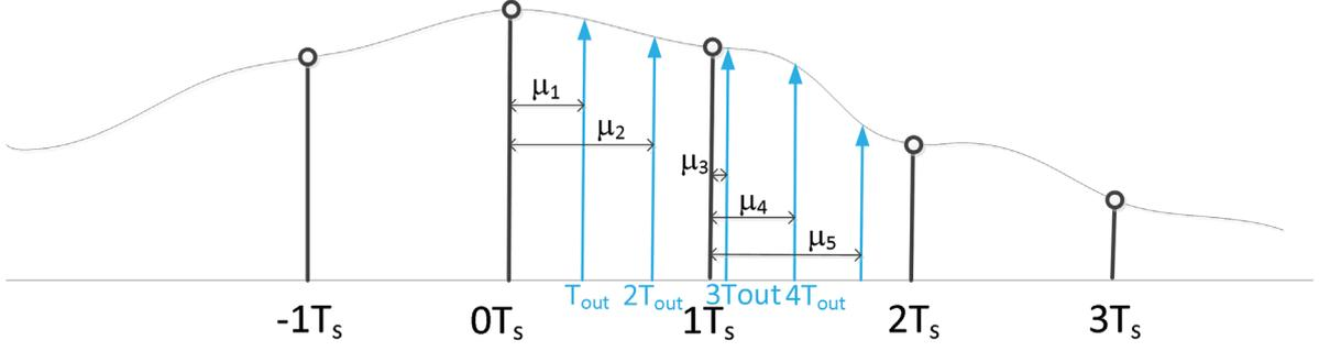
Figure 13: Illustration of Farrow interpolation resampling
