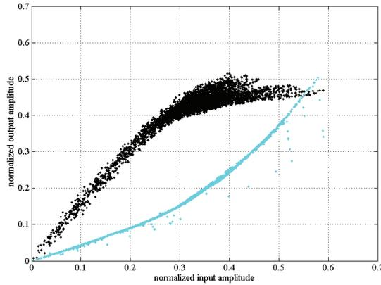
Figure 7: Measured AM/AM characteristics of PA (black) and of DPD (cyan).
