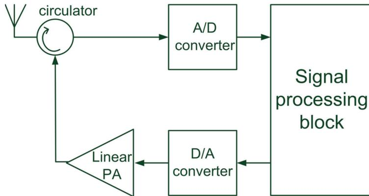
Figure 4: Basic concept of a software radio
