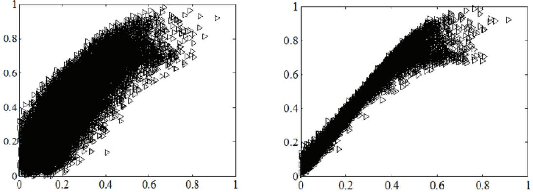
Figure 15: AM/AM without (left) and with (right) fine delay estimation
