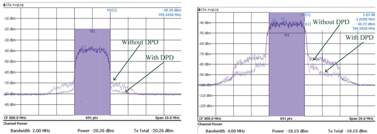
Figure 8: Spectra of the PA output without and with predistortion for 16-QAM (left) and LTE (right) signals.
