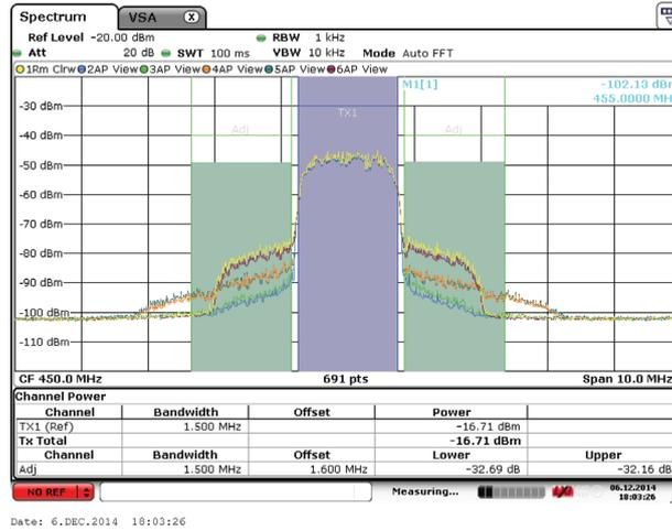
Figure 12: Power spectrum for example PA in 450 MHz band: TR1 - yellow is PA without DPD, TR2 - blue curve denotes DDR2 DPD ( $K = 11$ ,  $Q = 0$ ), TR3 - green color is PA with DDR DPD ( $K = 7$ ,  $Q = 0$ ), and TR4 - orange trace is DDR2 DPD ( $K = 3$ ,  $Q = 0$ ), TR5 - dark green is DPD with LUT (cubic interpolation) and TR6 - purple is PA without DPD for different output power.
