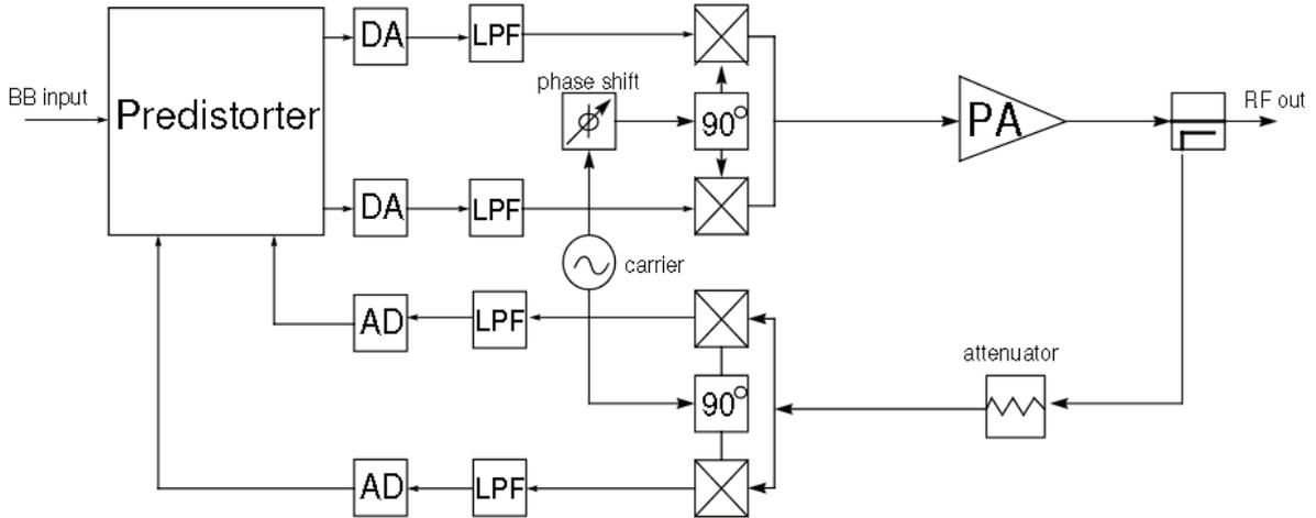
Figure 1: Digital predistortion principle.
