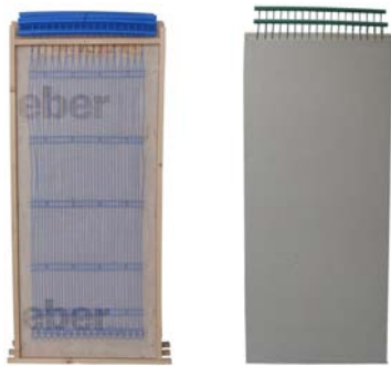
Figure 2.14: Photograph of the experimental TABS. Left: the TABS before the application of the plaster, right: the complete TABS [34]
