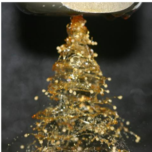
Fig. 7.5 Suspension structure at low pressure and low GLR, nozzle with moderate swirler (I).
