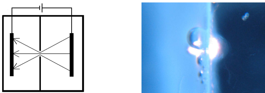
Figure 1. Left: Simplified scheme of the pin-hole configuration in the DC voltage regime. Arrows represent a vector of the applied electric field in the DC regime. Right: Photograph of plasma channels propagating from the pin-hole in the dielectric barrier towards the cathode (on the left side of the barrier) and towards the anode (on the right side of the barrier).
