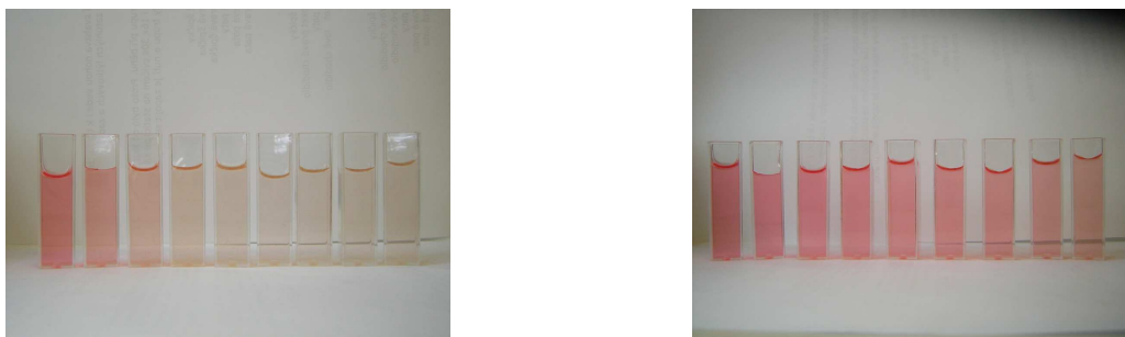
Figure 12. Samples of DR79 solution treated by the DC pin-hole discharge: anode (left) and cathode part (right); initial dye concentration of 12 mg/L, NaCl electrolyte, initial conductivity of 500 \mu\text{S}/\text{cm} , PET dielectric barrier (thickness of 0.25 mm), central pin-hole (diameter of 0.25 mm), electrode distance of 2 cm with respect to the barrier, input power of 160 W.
