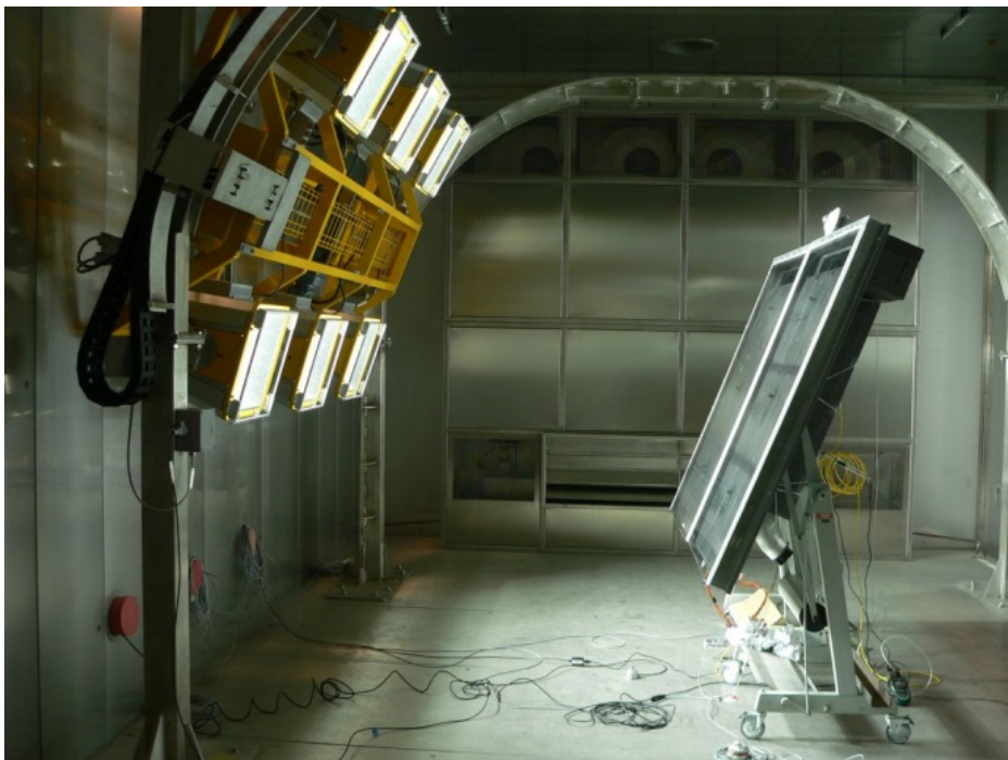
Fig. 9 Experimental collectors in the climatic chamber
