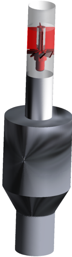
Figure 4.1: Sudden expansion chamber with swirler [12]
