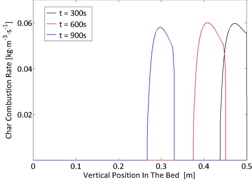
Figure 11: Propagation of char combustion reaction front as predicted by the variable-porosity model for 20-mm particles.
