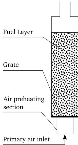
Figure 2: Schematic diagram of an experimental reactor.
