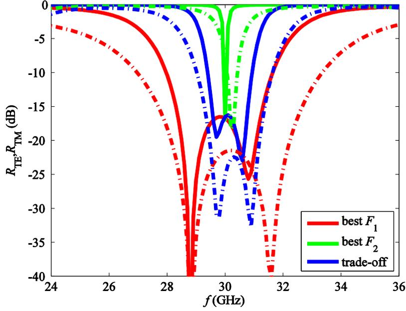
**Fig. 4.3:** Reflection coefficient TE (solid line) and TM (dashed) for three band-pass filters designed by MOSOMA: red line (the best solution according to  $F_1$ ), green (the best  $F_2$ ) and blue (trade-off) [PK 7].
