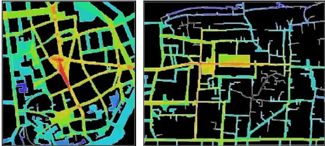
Figure 1: The Visibility Graph Analysis (VGA map) of the study area, points marked with the red colors refers to the most integration values, and the dark blue to the least, (left) area of Brno Center, (right) Old Damascus.
