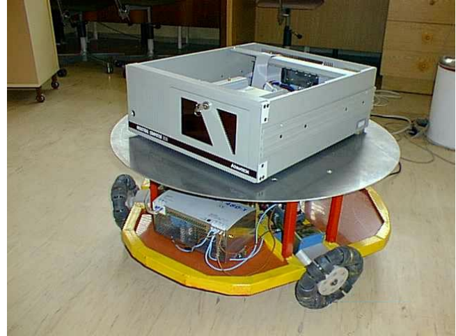
fig. 3 Omnidirectional undercarriage with three wheels
