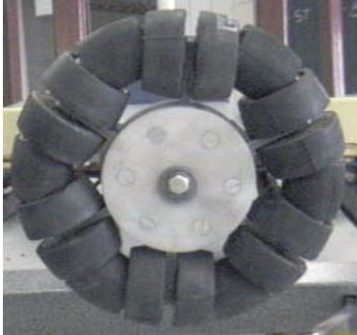
fig. 2 special omnidirectional wheel
