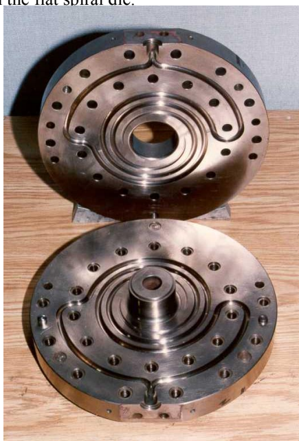
Fig. 2 Typical flat spiral distribution system.
