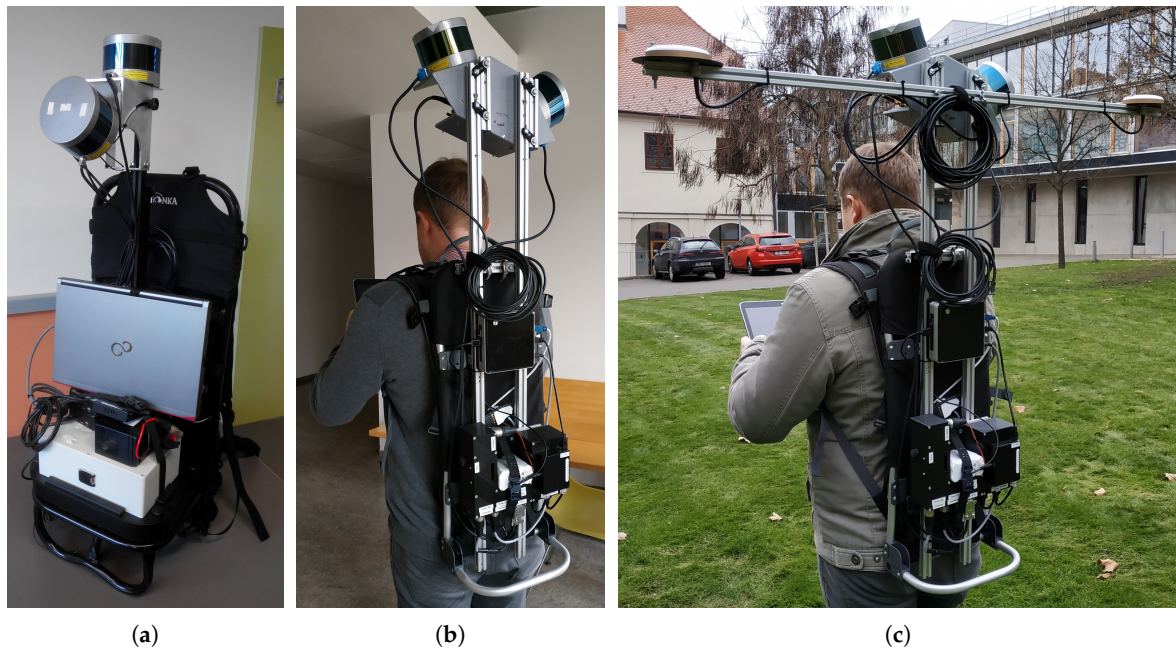
Figure 7. The initial (a) and improved (b,c) prototype of our backpack mapping solution for both indoor (b) and outdoor (c) use. The removable dual GNSS antenna provides precise heading information, aiding for outdoor odometry estimation and also georeferencing of the resulting 3D point cloud model. It should be noted that the position of LiDAR scanners is different in the initial and the later solution. This is elaborated on in the next section.
