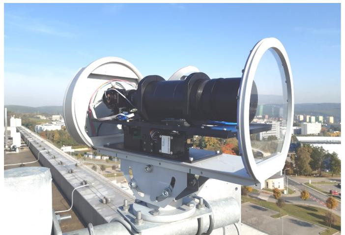
Fig. 1: 3D model and the optical assembly during tests.
