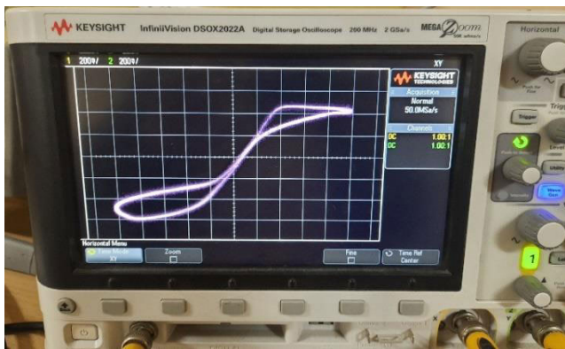
FIGURE 24. Pinched hysteresis loop of meminductor circuit obtained at the frequency 400 kHz.
