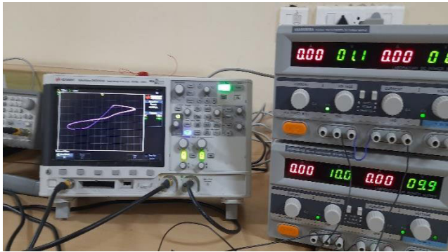
FIGURE 23. Pinched hysteresis loop of memcapacitor circuit obtained at a different frequency 400 kHz.
