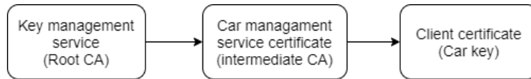
Fig. 3. A certificate chain reflecting the mode in which the key management service can be autonomous, instead of being a part of the car sharing or fleet management system.
