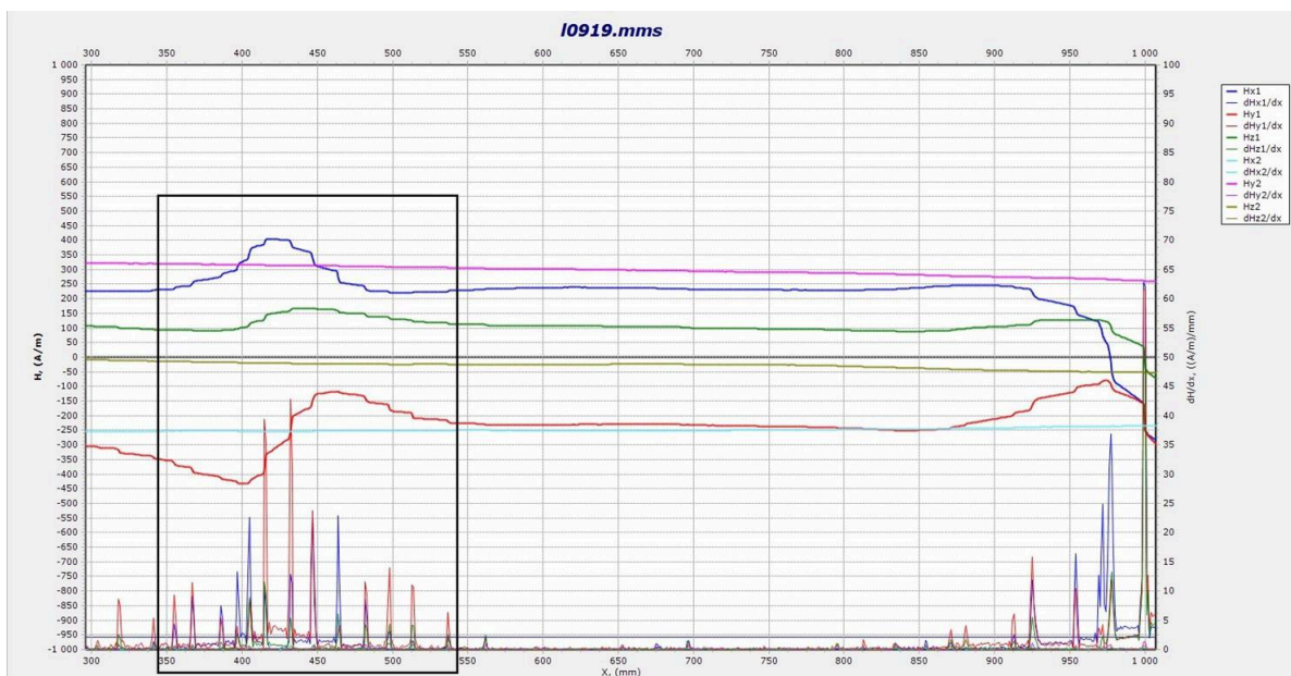
Figure 10. Magnetogram 109169.mms correspond to strand L96 – after 6 hours of corrosion process
