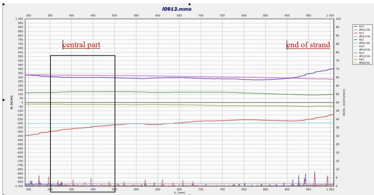
Figure 8. Magnetogram 10913.mms corresponds to undamaged steel strand L90
