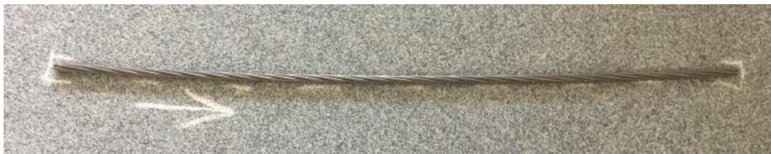
Figure 7. Intact steel strand L90
