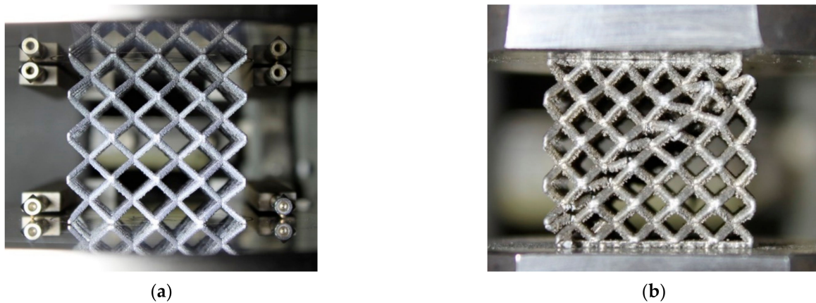
Figure 3. (a) The principle of the displacement measurement during the compression test. (b) Collapse phase of the BCC lattice structure during the compression test.
