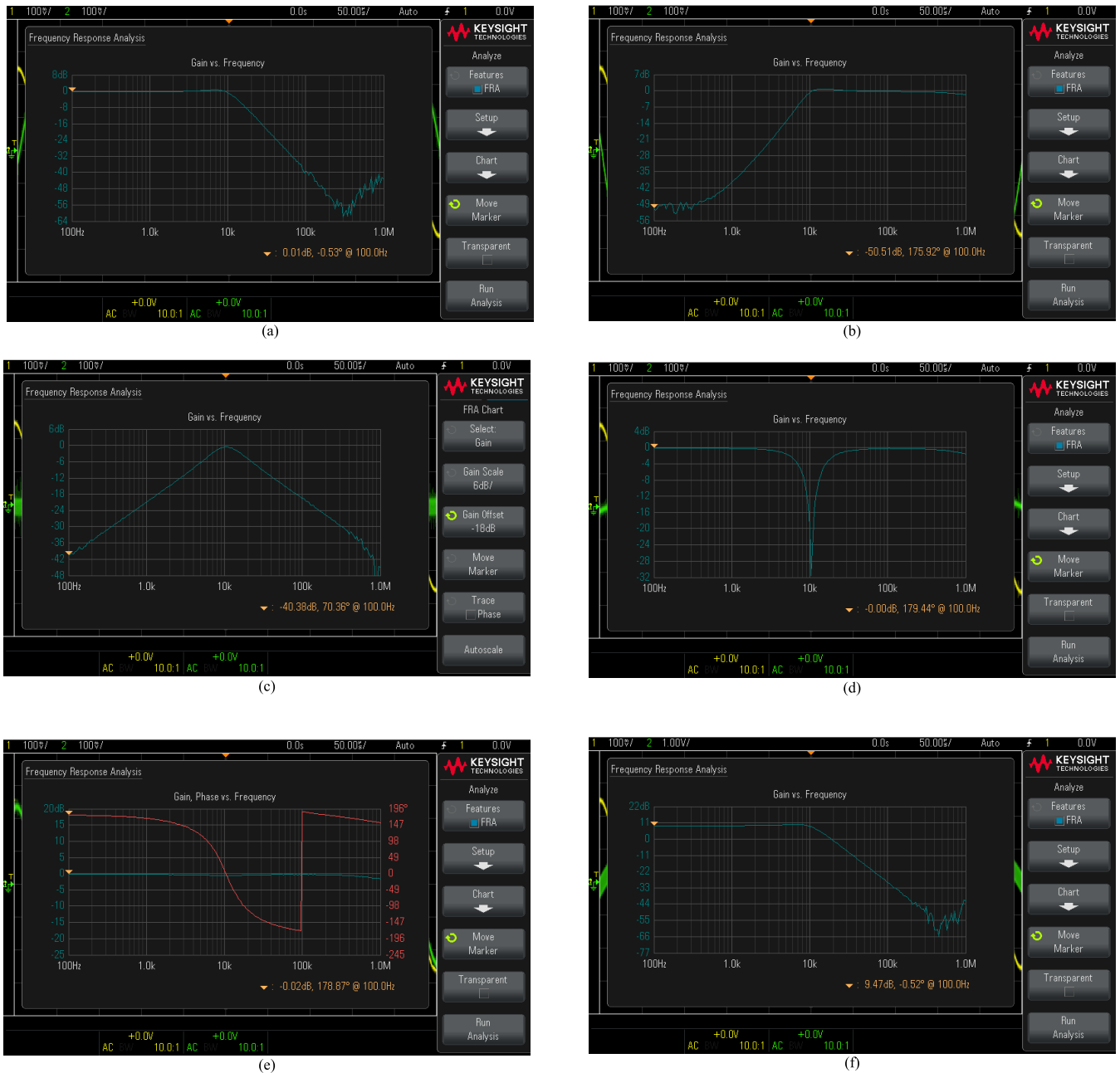
FIGURE 28. Measured frequency responses, a) LPF, b) HPF, c) BPF, d) BSF, e) APF and f) LPF with voltage gain greater than unity.
