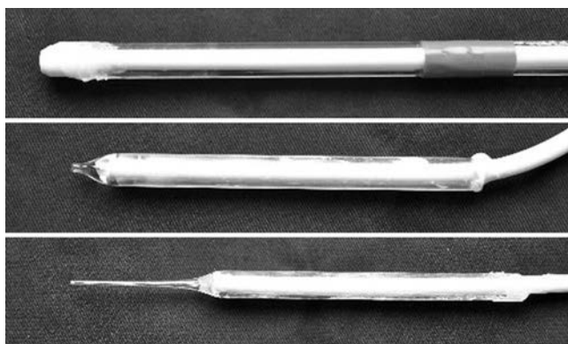
FIGURE 3.16 Practical realization of the pinhole-based electrodes for the surface cleaning of ancient objects. Electrode with alumina ceramic head (top), fully quartz made electrode (middle), tiny quartz made electrode for the treatment in holes (bottom). The diameter of the glass part is 10 mm in all cases.
