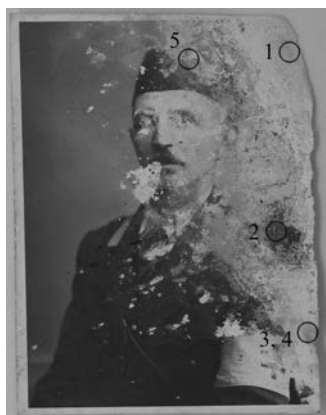
FIGURE 6.2 Historical photography. Individual sampling on photography: 1 – scalpel, 2 – swab, 3 – adhesive tape, 4 – adhesive tape, 5 – swab.
