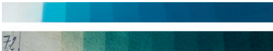
FIGURE 8.7 Sample of cyanotype with different optical density ( D_0=0.1 - 2.1 ) before aging (picture above) and after aging 72 h in the Q-SUN chamber (photo was taken 3 h after removal from the Q-SUN chamber – picture below; Grešová 2019).
