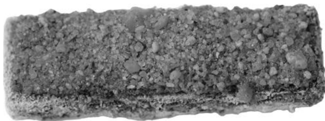
FIGURE 8.20 Iron sample corroded in HCl vapor with sandy incrustation.
