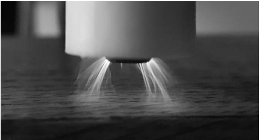
FIGURE 3.22 Piezoelectric plasma pen activating surface of the wood.
