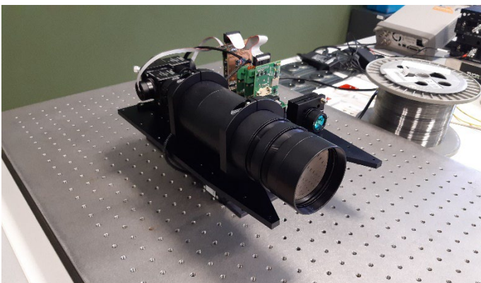
Obr. 1: The OWC unit (left) and the fiber stabilization and evaluation unit (right) for the transmission of optical frequency.
