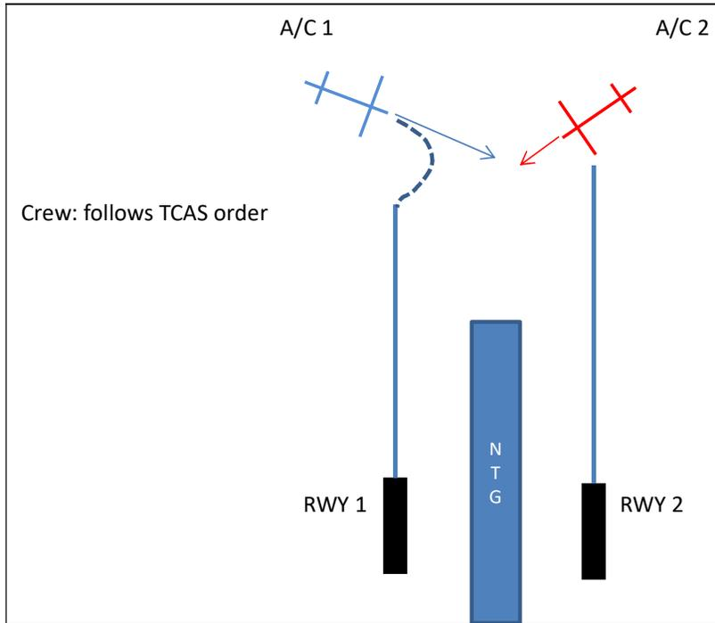
Figure 7 : Alert when joining the final approach path
