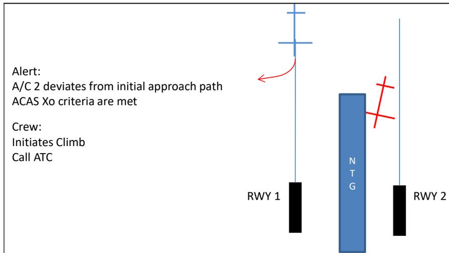
Figure 8 : Alert during CSPO-3000 approach
