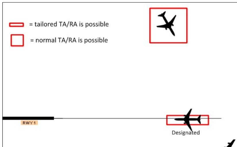
Figure 5: CSPO-3000 mode illustration (source: FAA, RTCA SC-147)
