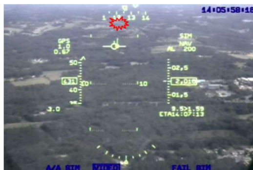
Figure 9: Example of aircraft visibility, T0 - 4,64 s (distance between aircraft : 1 276 m)
