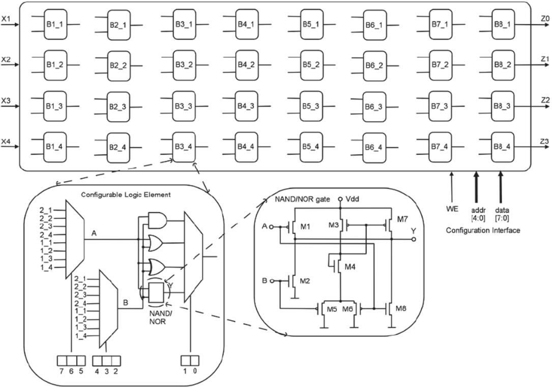
Fig. 1: The REPOMO32 chip, iplementation details of the CLE block and NAND/NOR gate
