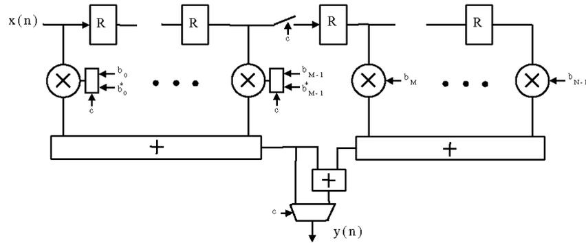
Fig. 2: Circuit Structure of Polymorphic FIR Filter
