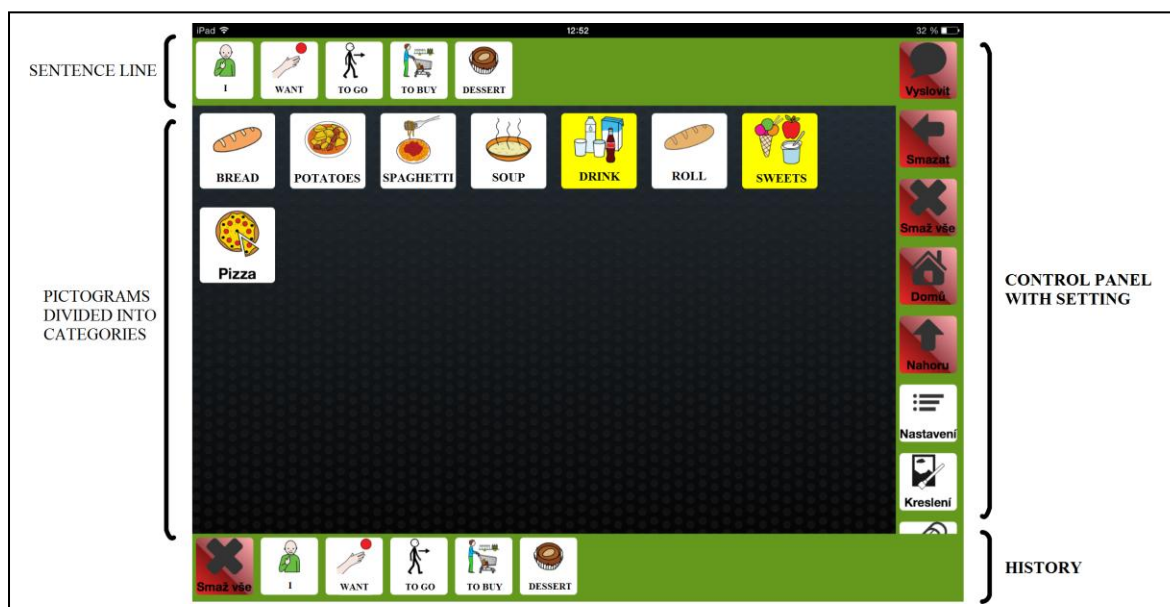
Figure 1. Easy-Talk application working desktop. Category and pictogram selection area is separated by different visual boarding. Categories are separated from proper pictograms by yellow background (customisable). Control panel is sliding. Beside navigation control panel contains SETTING button, DRAWING CANVAS and TEXT INPUT buttons.
