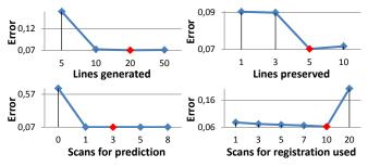
Fig. 9: Tuning of the registration parameters. Values of the lowest error (16) are highlighted in red. Graphs show the error trend based on the number of lines generated and preserved in the each polar bin, the number of previous registrations used for prediction and the number of frames used for multi-scan approach.
