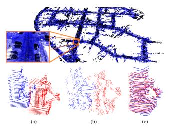
Fig. 1: Top: The environment map created by merging previously registered Velodyne point clouds. Bottom row: An example of the registration process. Two unaligned scans (a), sampled by line segments to produce *line clouds* (b) which are further used to estimate resulting alignment (c).
