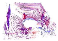
Fig. 2: Point clouds captured by the Velodyne LiDAR scanner and associated issues. The ring structures fit to each other for unregistered data (left) which disables the convergence of typical ICP approach to proper registration. The data is also sparse, causing lack of spatial correspondences between scans. See the well registered scans (right) - most of the points on floor in blue scan have no proper correspondence in red scan
