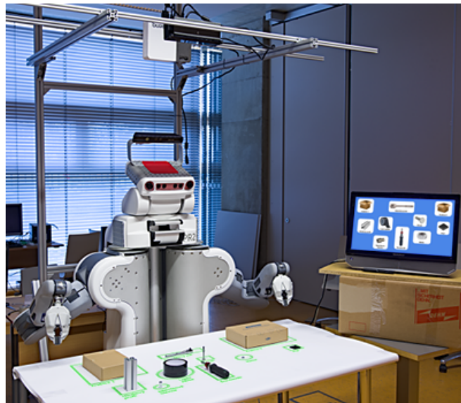
Fig. 1: Prototype of the human-robot shared-space environment with augmented reality user interface (image edited).
