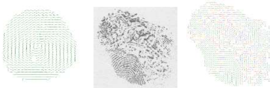
Figure 6. Examples of Orientation Estimation Images (Healthy Fingerprint, Fingerprint Affected by a Skin Disease, Detected Damaged Areas)
