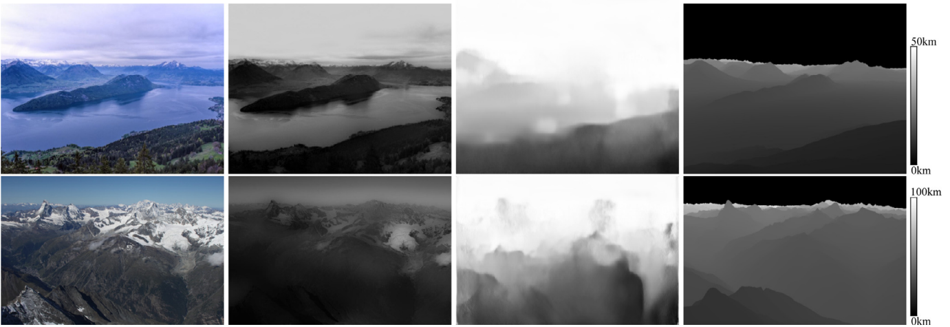
Fig. 5. Given a single color input image, our system creates more plausible absolute depth maps (right) unlike previous depth map estimations (e.g., dark channel prior [48], or deep learning based method [63]; middle).
