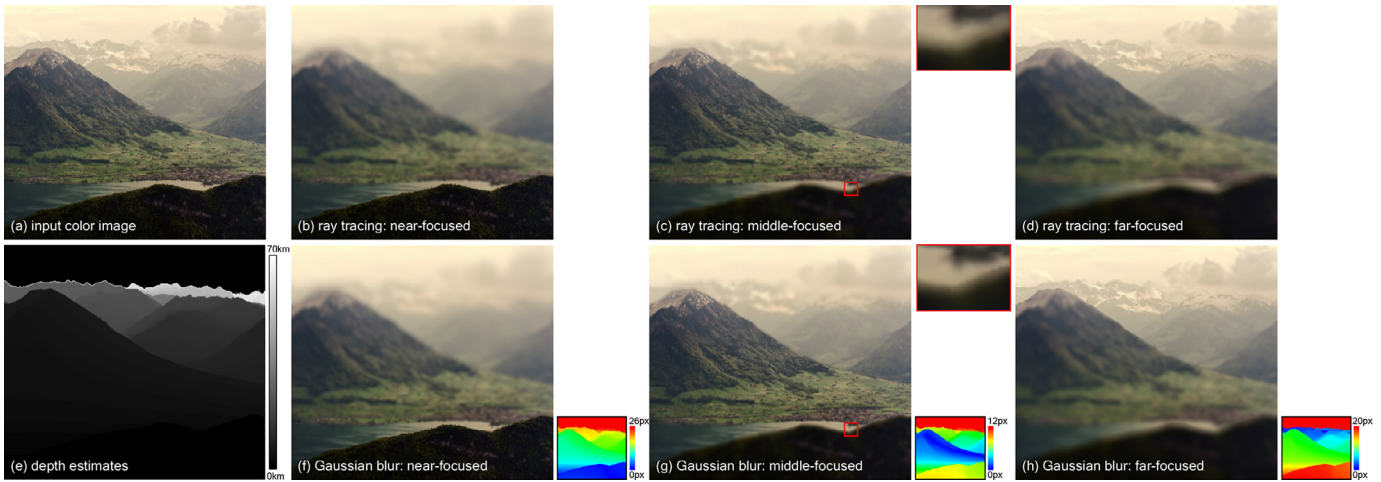
Fig. 12. Comparison of ray-traced defocus blur (b–d) and Gaussian blur (f–h) generated from the color (a) and depth inputs (e). The black-edged boxes show blur kernel sizes (in pixels). The ray tracing better handles discrete depth boundaries than Gaussian blur does (see the red insets).
